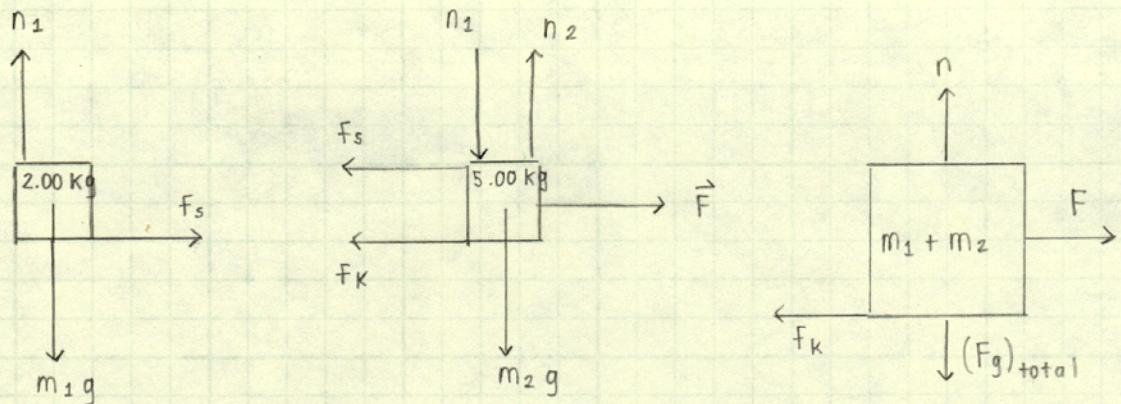
The force of static friction between the blocks accelerates the 2.00 kg block.
