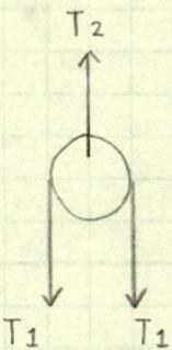
$$\begin{aligned} F &= T_2 - 2T_1 \\ F &= ma = 0 \\ T_2 - 2T_1 &= 0 \\ T_2 &= 2T_1 = 2mg \\ T_2 &= 2(5.00 \text{ kg})(9.80 \text{ m/s}^2) \\ T_2 &= 98.0 \text{ N} \end{aligned}$$
