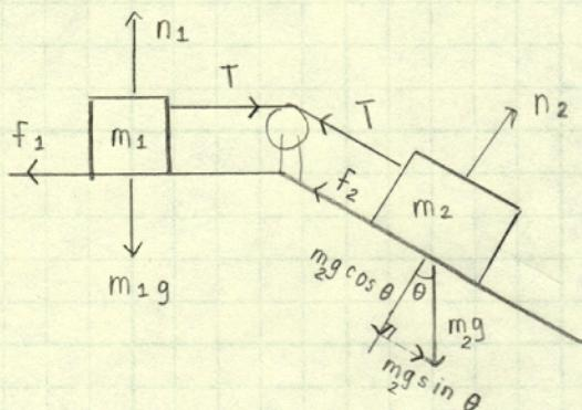
For the system to start to move, the force tending to move m<sub>2</sub> down the incline, m<sub>2</sub>g sin θ, must exceed the maximum friction force.
