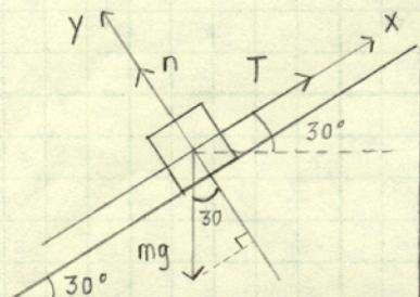
$$\begin{aligned} \text{x-component} \\ T - mg \sin 30^\circ &= 0 \\ T &= mg \sin 30 = (5.00 \text{ kg})(9.80 \text{ m/s}^2) \sin 30 \\ T &= 24.5 \text{ N} \end{aligned}$$
