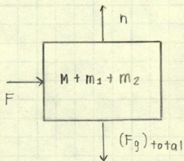
normal forces are always  $\perp$  to the contacting surfaces
