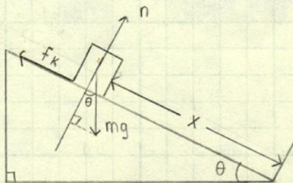
$$\begin{aligned} \text{y-component} \\ n - mg \cos \theta &= 0 \\ n &= mg \cos \theta \end{aligned}$$
