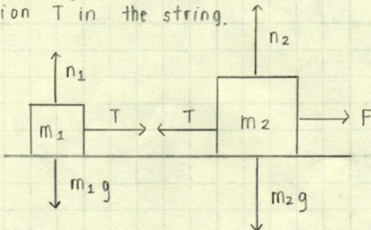
$$\text{x-component} \quad \text{For } m_2: F - T = m_2 a \quad (1)$$
