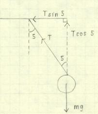
(b) x-direction  $T \sin 5^{\circ} = mar$   $a_r = \frac{T \sin 5^{\circ}}{m} = \frac{(787 \text{ N}) \sin 5^{\circ}}{80.0 \text{ kg}}$   $a_r = 0.857 \text{ m/s}^2$
