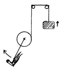
Since the wheel is round, the lever arm for the weight stack does not change as the leg goes through its motion. So the leg exerts the same force throughout the motion.
