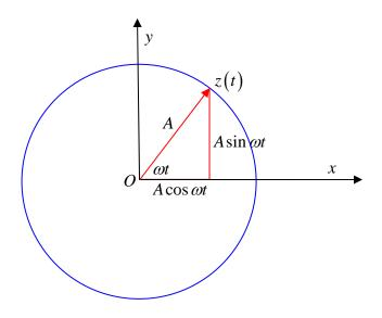
The angular velocity is  $\omega$ , the actual velocity in the complex plane is dz(t)/dt.
