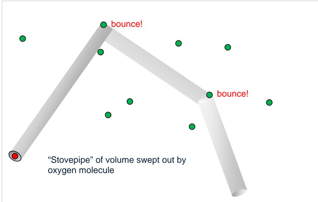
If the density of the nitrogen is  $n$  molecules per cubic meter, the number of  $\text{N}_2$ 's in this stovepipe volume will be  $\pi d^2 L n$ , in other words, this will be the number of collisions. Therefore, the average distance *between* collisions, the mean free path  $l$ , is given by:
