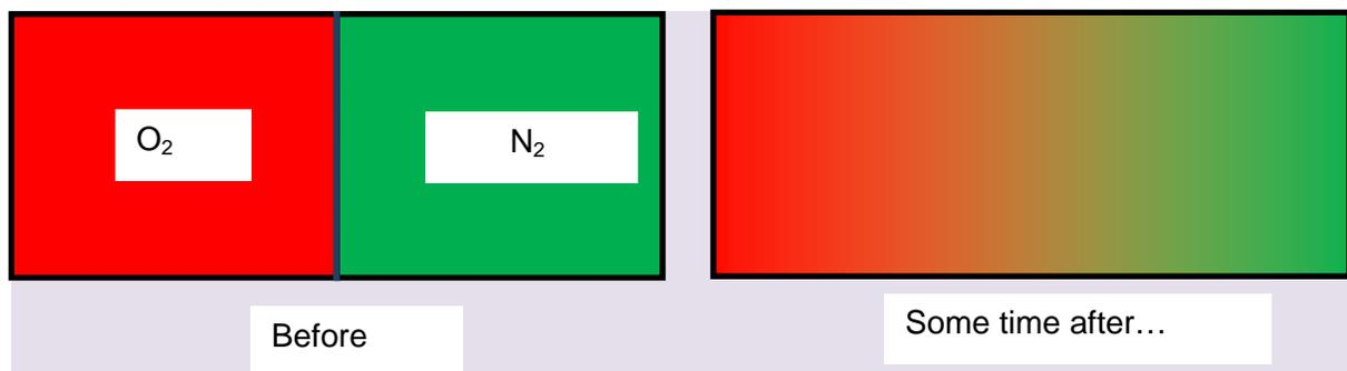
For a box holding a few liters, it takes of the order an hour or so for the gases to mix. (We're assuming the temperature is kept constant so that convection currents don't arise—such currents would reduce the time substantially.) Obviously, the rate of mixing must depend on the mean free path: if it was centimeters, the mixing would be pretty complete in milliseconds. In fact, as we shall see, the mean free path can be deduced from the measured rate of penetration of one gas by the other.
