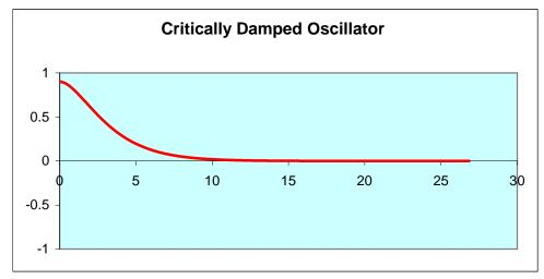
This corresponds to  $\omega' = 0$  in the equation for x(t) above, so it is a purely exponential curve. Notice that the oscillator moves more quickly to zero than in the overdamped (stiff oil) case. You might think that critical damping is the best solution for a shock absorber, but actually a little less damping might give a better ride: there would be a slight amount of bouncing, but a quicker response, like this:
