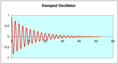
The yellow curves in the graph above are the pair of functions  $+e^{-bt/2m}$ ,  $-e^{-bt/2m}$ , often referred to as the *envelope* of the oscillation curve, as they "envelope" it from above and below.
