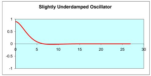
You can find out how your shock absorbers behave by pressing down one corner of the car and then letting go. If the car clearly bounces around, the damping is too little, and you need new shocks.
