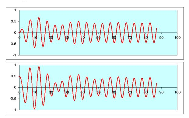
Notice that after about 70 seconds, the two curves are the same, both in amplitude and phase.
