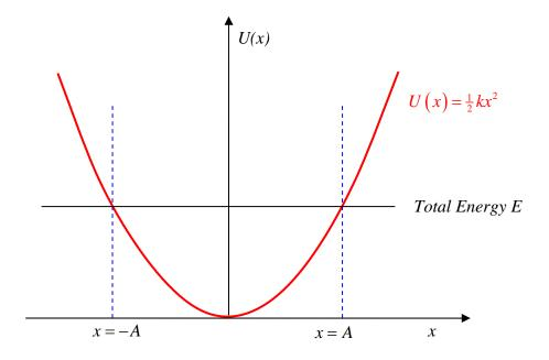
Potential Energy U(x) for a Simple Harmonic Oscillator. For **total** energy E, the oscillator swings back and forth between x = -A and x = +A.
