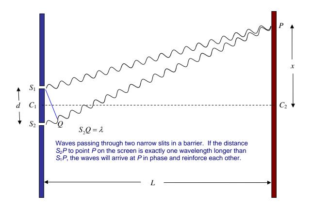
On the other hand, at a point approximately half way from the center of the screen to *P* the waves from the two sources will arrive at the screen exactly *out* of phase: the crest of one will arrive with the trough of the other, they will cancel, and there will be no light. Evidently, then, we will see on the screen *a series of bright areas and dark areas*, the brightest spots being at the points where the waves from the two slits arrive exactly in phase.
