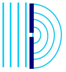
A plane wave encounters a barrier with an opening smaller than a wavelength: the wave spreads in circular fashion on the far side.
