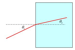
**Snell's Law** : a ray of light entering glass from air is bent towards the normal, and  $\sin \theta_1 / \sin \theta_2$  is the same for any entering angle.
