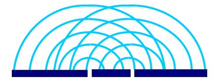
Waves spreading out from two small slits in a barrier: the blue circles represent wave crests, where two cross the wave has maximum positive value, for example along the central line.
