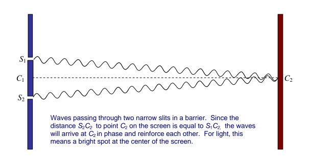
For light waves passing through two narrow slits and shining on a screen (on the right) there will be another bright spot at a point P away from the center  $C_2$  of the screen, provided the distances of P from the two slits differ by a whole number of wavelengths:
