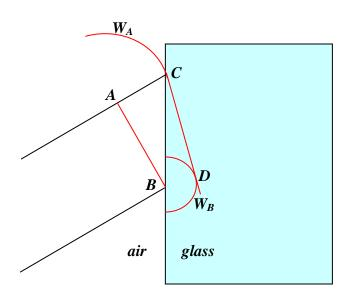
Huygens' explanation of refraction: showing two wavelets from the wavefront AB:
