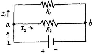
Two resistors in parallel  $\therefore \Delta V_1 = \Delta V_2 = \Delta V$
