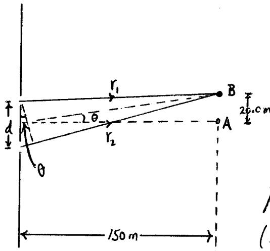
$$r_1 - r_2 = d \sin \theta, \lambda = 3.0 \text{ m}$$
