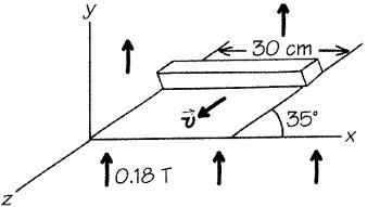
conducting loop. The plane of the rails makes an angle of 35 degrees with the horizontal, and a uniform vertical magnetic field of 0.18 T, pointing upward, exists throughout the region. What is the steady speed of the wire?
