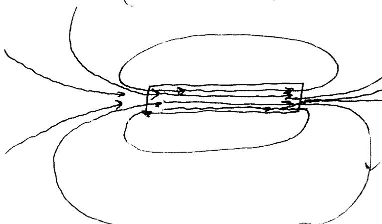
Note that the field lines leaving the iron are close together, adding strongly to the local field... but alongside the metal they extend over all space, having very little effect at any given place.
