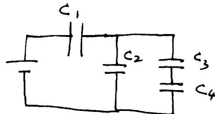
Thus,  $C_3$  and  $C_4$  are in series:  $C_{34} = \frac{C_3 C_4}{C_3 + C_4} = \frac{2 \times 5}{2+5} = \frac{10}{7}$
