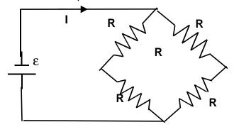
This circuit is clearly equivalent to two resistors of value 2R which are in parallel. Therefore the final equivalent resistance is R.
