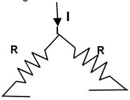
In order to complete the circuit what we have to connect to the points a and b are exactly identical in other words looking down from a and b the circuit looks the same. Therefore the potentials a and b are identical. This means that no current can flow along the diagonal connection and the resistor there need not be included at all. Thus the circuit simplifies to:
