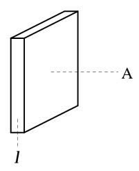
We must supply to that volume of air an energy  $\Delta E = \frac{1}{2}mv^2$ , and the time in which we have to supply that energy is the time it takes for that volume to pass by the fan which is  $\Delta t = \ell/v$ . Therefore, the power, which is energy per time, is
