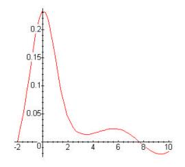
A trick for estimating ground state energies in wells is to approximate the potential well V(x) near its minimum  $x_0$  by a Taylor expansion to order  $(x - x_0)^2$ . In this particular case,  $x_0 = 0$  and one would have  $V(x) \approx x^2$ . With this approximation we have the Schrödinger
