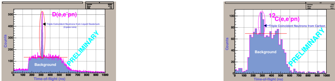
Figure 28: Shown on the left is the coincidence time spectrum from the over-determined D(e, e'pn) reaction. Shown on the right is the coincidence time spectrometer for the ^{12}\text{C}(e, e'pn) reaction.
