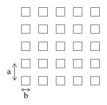
6. Suppose a screen as in Problem 5 has a = 0.5 mm, b = 0.1 mm, and is illuminated with light having  $\lambda = 500$  nm. The screen is the object of an imaging system as shown, where the lens focal length is f = 100 mm. A square hole with side p is placed in the focal plane of the lens so as to low-pass filter the image. What value of p should be used to give a smooth, uniform image with no modulation from the screen pattern? (You can assume here that  $N \gg 1$ .)
