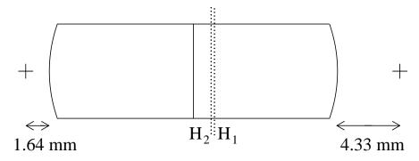
Principle planes separated by 0.2 mm system acts almost exactly like thin lens
