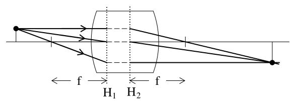
Draw diagram just like thin lens but rays skip across between principle planes
