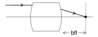
Back focal length = distance from back vertex to back focal point
