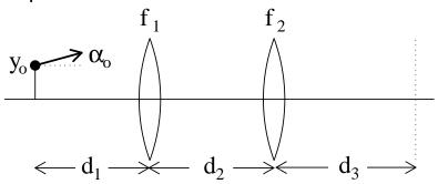
Consider ray starting at object:  $\mathbf{v}_o = \left[ \begin{array}{c} \alpha_o \\ y_o \end{array} \right]$
