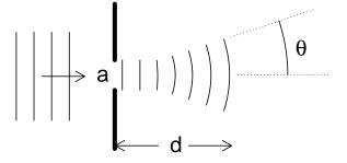
For  $\theta d \ll a$ , diffraction not significant use ray optics
