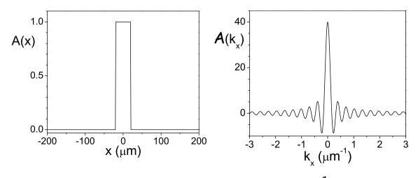
Filter cuts off  $|k_x| > ka/2f = 0.23 \ \mu m^{-1}$ approx at first zero of A
