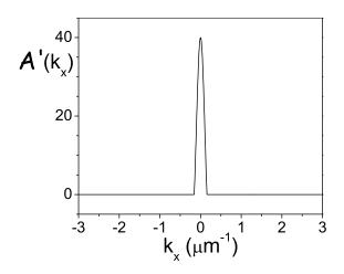
At image plane, get inverse transform of  $\mathcal{A}'$ = image of A, missing high  $k_x$  components
