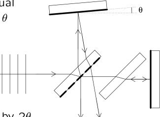
Output beams tilted by  $2\theta$
