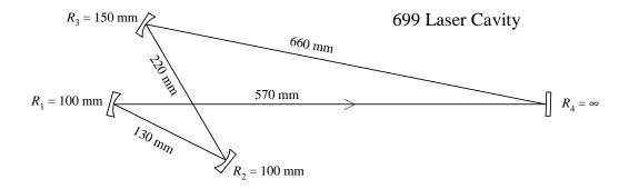
6. What is the longitudinal mode spacing of the 699 cavity, in MHz?
