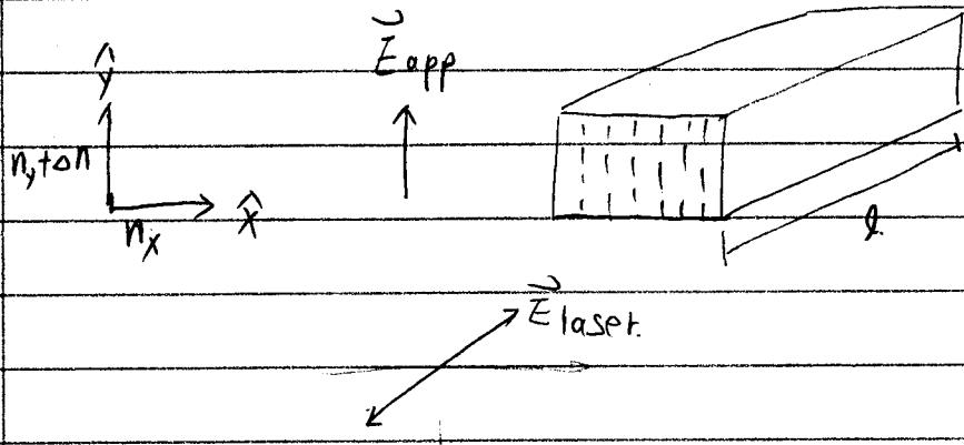
Send laser through crystal with polarization at  $45^\circ$
