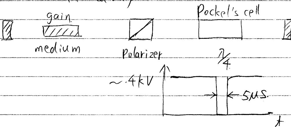
Normally, the high voltage applied on Pockel's cell makes it work as a quarter-wave plate.
