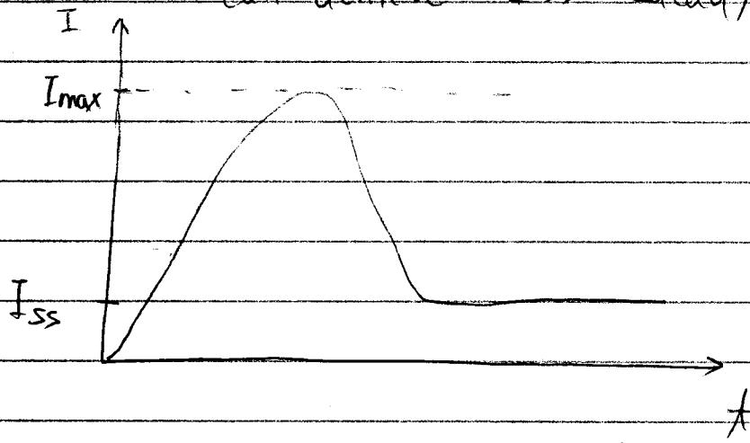
"Atoms give up energy faster than energy leaves cavity  $\rightarrow$  excess builds-up."
