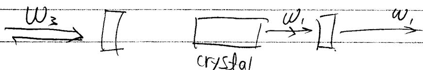
The eigenmode of the cavity, whose frequency has the right phase-match, will start oscillate (OPO).
