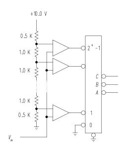
The speed of the ADC is of some interest when converting a time-varying signal to digital form. For example sounds in the audio range—speech or music, for example—are typically complex waveforms with frequency components up to 20 KHz. A basic criterion (Nyquist) states that in order to represent
