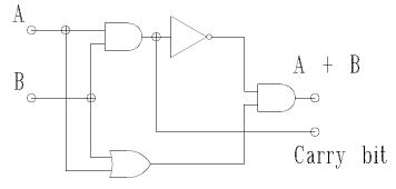
next column, as we do when adding by hand. If we AND the two inputs at the same time we XOR them, we obtain a carry digit (bit) only when both inputs are 1, which is what we want. Note we do not need an extra AND gate for this, the signal we need can be found after the first AND, as shown to the right.
