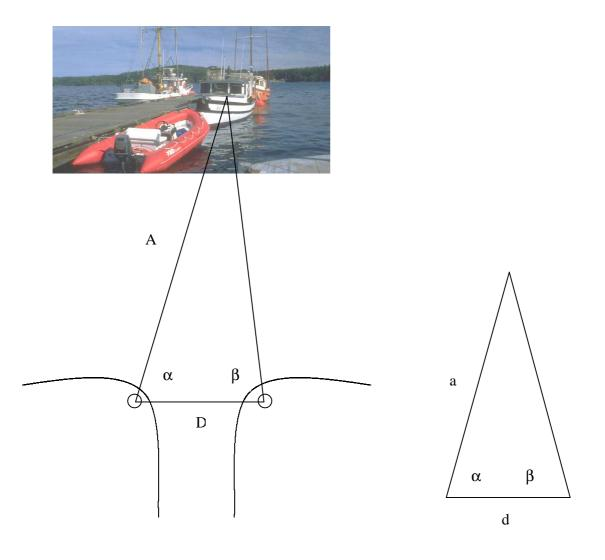
The drawn triangle is similar to the triangle created by the lines of sight of the observation post observers. This means the two triangles have the same shape; they just differ in size. The size difference can be enormous, that makes no difference. The shapes are the same, and so the ratios of corresponding sides must be the same. That means:
