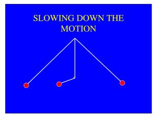
He then built a modified pendulum as shown above. A peg is inserted below the suspension point, so as the weight swings past it, the peg suddenly shortens the length of the pendulum causing it to swing up abruptly. What he found is that it still rises to the same height as before, and does so again back on the other side. Galileo argued that this shows that a falling pendulum reaches the same speed at the bottom of its motion regardless of how steep the descent was.
