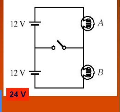
Follow-up: What happens if the bottom battery is replaced by a 24 V battery?
