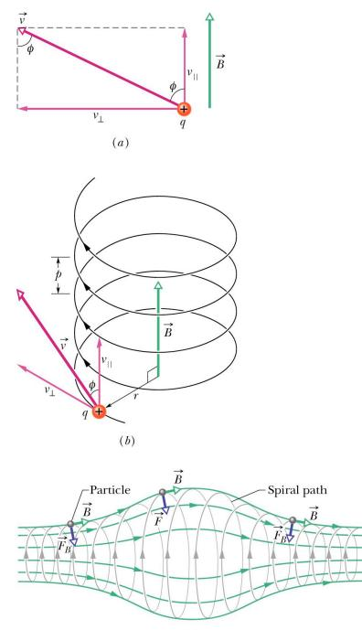
Magnetic bottle. The charge is trapped inside and spirals back and forth Torques on current loops
