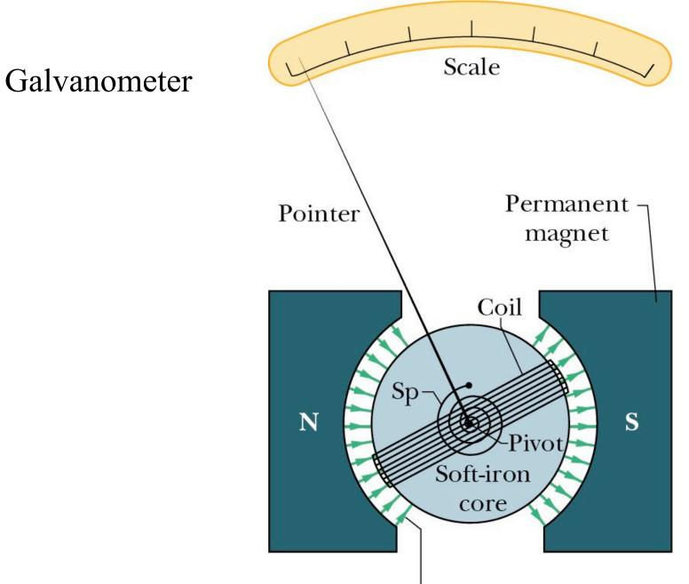
Uniform radial magnetic field Magnetic dipole moment  $\mu$
