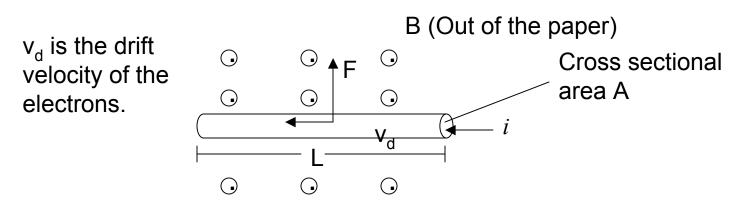
When a wire carries current in a magnetic field, there is a force on the wire that is the sum of the forces moving charges that carry the current.
