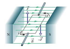
Above is a rectangular loop of wire of sides *a* and *b* carrying current *i*. B is in the plane of the loop and  $\perp$  to *a*.
