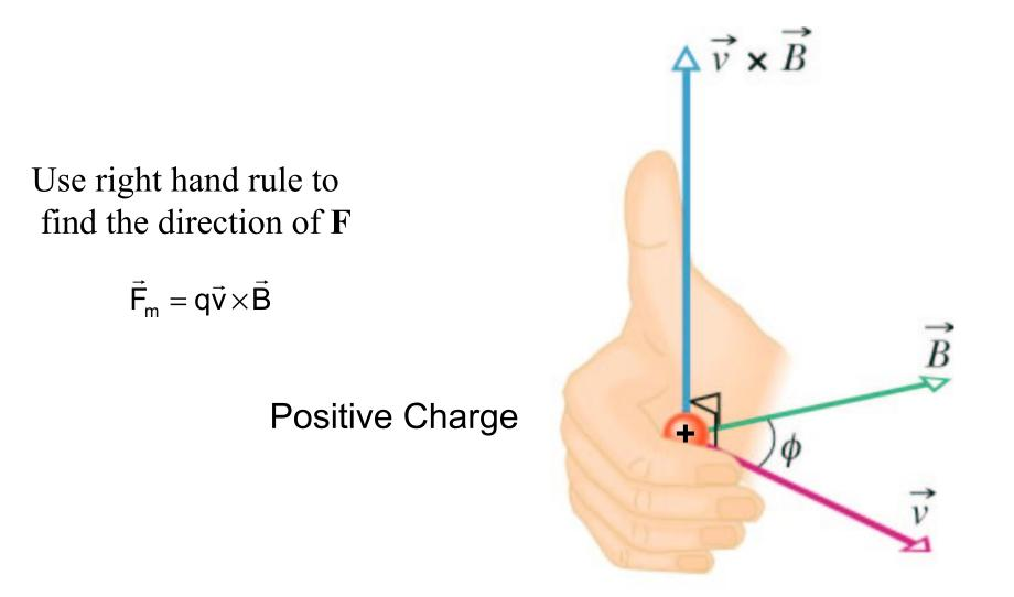
Rotate **v** into **B** through the smaller angle  $\phi$  and the force **F** will be in the direction a right handed screw will move.
