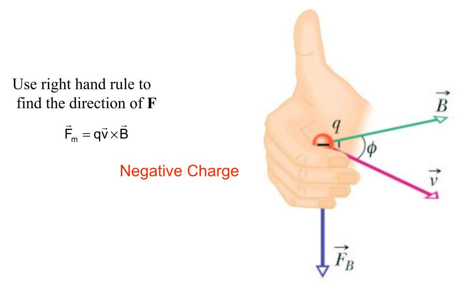
Rotate **v** into **B** through the smaller angle  $\phi$  and the force **F** will be in the opposite Direction a right handed screw will move.
