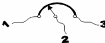
Figure 5-3: Schematic of a potentiometer. As the dial is rotated, the amount of resistive material between terminals 1 and 2, and between 2 and 3, changes. Thus it is a variable resistor.
