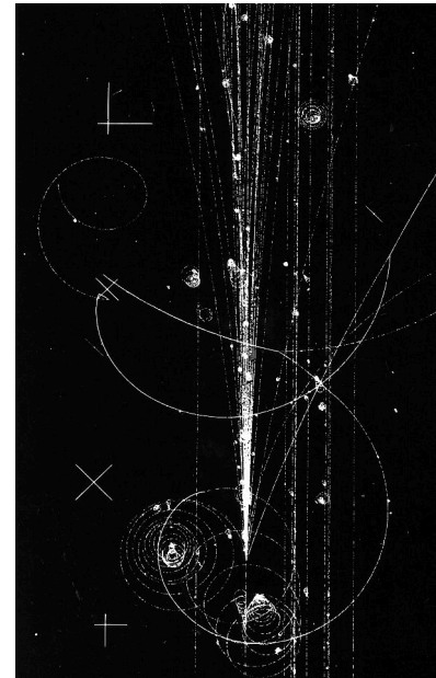
Figure 3: Traces of charged particles in a bubble chamber at Fermilab (1973).
