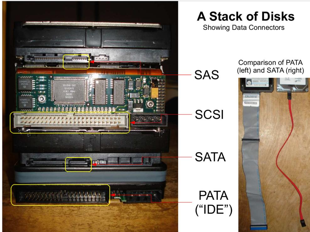
Here are four different types of disks, all of the same width. Each is a standard “3.5-inch” disk, and would fit into the same slot as any of the others. The two most common types of disks are Parallel ATA (PATA) disks (sometimes loosely called “IDE” disks) and Serial ATA (SATA) disks. SATA is the successor to PATA, and is found almost universally in new computers.
