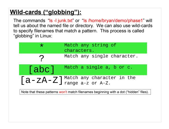
It's important to remember how wild-cards work on the Linux command line. If we type a command like "ls \*.txt", here's what happens internally:
