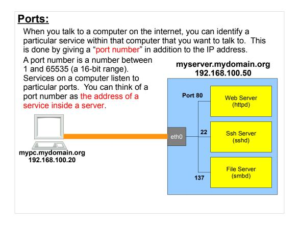
A port number is actually used at both ends of the connection. In the illustration above, the traffic leaving "mypc.mydomain.com" would originate from a particular source port on that computer. If the computer were browsing the web, for example, the traffic would originate from some randomly-assigned port on mypc, and would be address to destination port 80, on the remote computer, where the web server would be listening.
