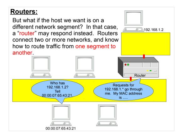
A network "segment" is a section of a network that is connected at the physical layer. Traffic can travel between all computers on the same segment without the help of routers or other intermediate devices that understand higher-level protocols.
