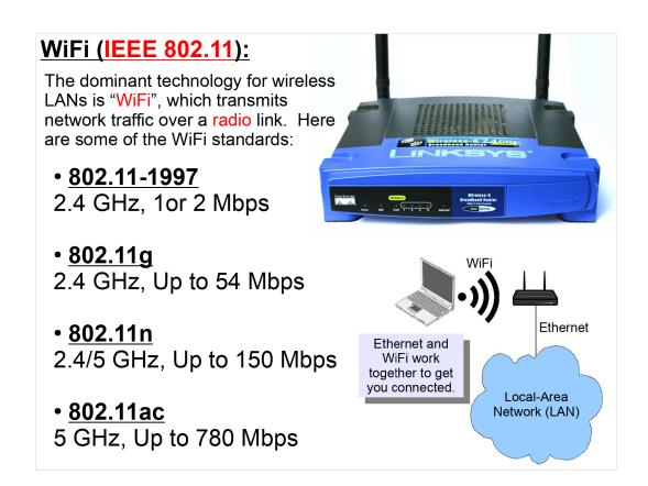
WiFi provides wireless connections to devices called Access Points. These access points are usually connected via Ethernet to the LAN. You could think of the wireless link as a way of wirelessly getting your laptop connected to the local Ethernet.
