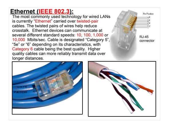
The connectors at the ends of the cables are called RJ-45 connectors. They're a type of modular connector similar to modular telephone connectors (called RJ-11), but wider.
