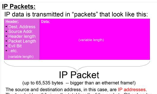
The source and destination address, in this case, are IP addresses. The "packet length" gives the total length of the packet. Other header entries give the length of the header itself, which can vary. The "Evil Bit" is an April Fool's joke. RFC 3514 proposes that an unused bit in the header be used to signify whether the sender is evil, making it easy to block malicious packets.
