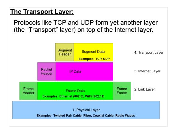
So now we have four layers in our layer-cake. On top of the physical layer, Ethernet frames carry data from computer to computer, guided by MAC addresses. Within those frames are IP packets, guided by IP addresses. Inside the IP packets are TCP or UDP segments/packets, addressed by port number.
