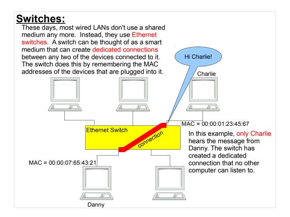
The switch does its work by remembering the MAC addresses of the devices that are plugged into it. For each connector, the switch maintains a list of the MAC addresses it has recently seen talking on that connection.
