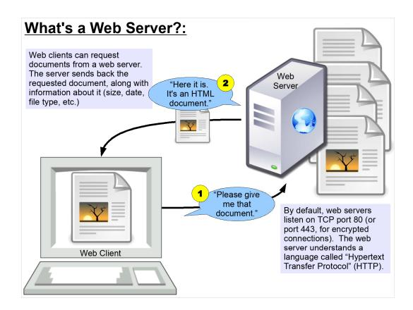
A web server is a computer that's capable of serving up documents through the "Hypertext Transfer Protocol" (HTTP). A network service running on these computers listens to TCP port 80 and/or port 443, and responds to HTTP requests.
