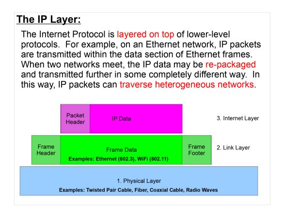
We're starting to build up a stack of protocols, each of which adds features unavailable at lower levels. The physical layer gives us a mechanism for transmitting zeros and ones. The "link" layer (e.g., Ethernet) gives us a way to send a set of zeros and ones to a particular computer. The Internet layer gives us a way to transmit data across a heterogeneous network. We'll add two more layers before we're done.
