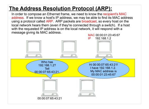
To broadcast a request on an Ethernet network, you send it to the special MAC address "FF:FF:FF:FF:FF:FF.".
