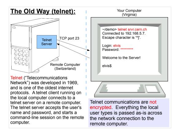
"rlogin" (sometimes invoked by "rsh") is similar to telnet. It also creates an unencrypted command-line connection to a remote computer.
