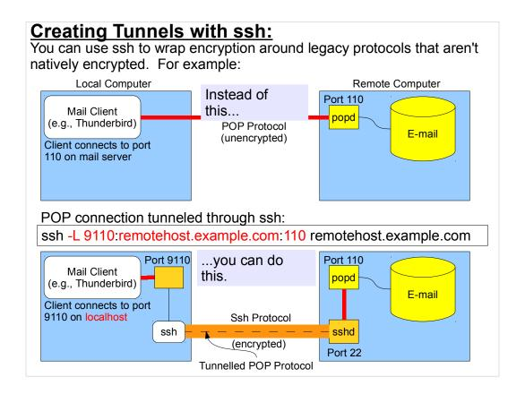
We've already talked about the special provisions in ssh that make it easy to create an encrypted tunnel for X connections. Here we see that this functionality isn't limited to X. It can be extended to any protocol.
