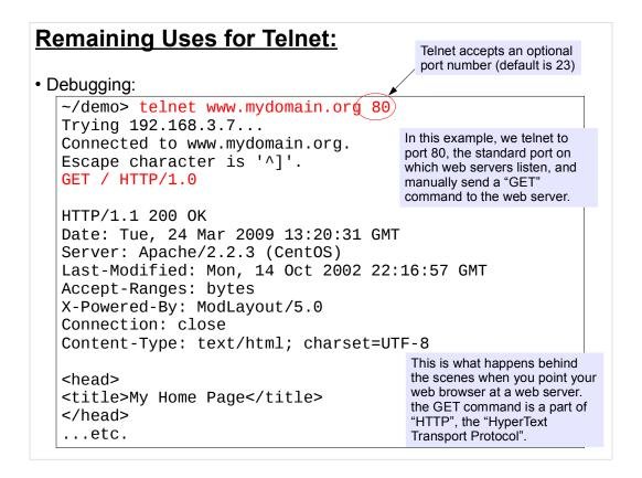
Telnet essentially gives you a (almost) raw TCP connection to a port on a remote computer. By default, telnet connects to port 23 (where the telnet server listens), but you can tell it to connect to any other port. This makes telnet useful for manually sending data to servers on remote computers.
