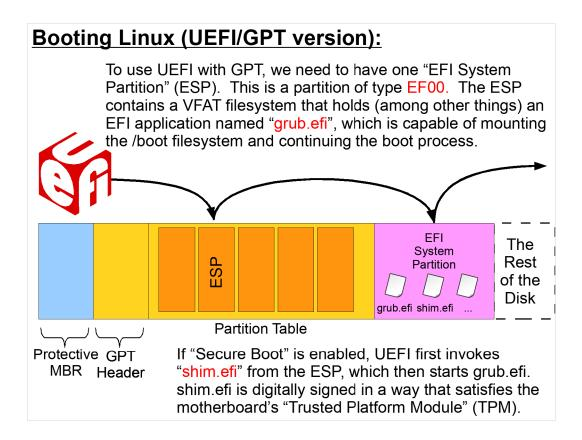
Finally, when we use UEFI instead of a BIOS, the UEFI processor is smart enough to read the partition table and mount a special filesystem. One or more of the EFI applications (e.g. grub.efi) in this filesystem is then run to continue the boot process.
