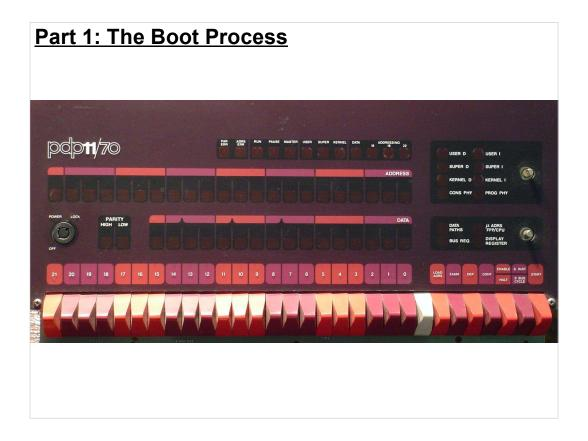
Once upon a time, computers like this PDP-11 were booted by flipping a set of switches, to enter a memory address, and then telling the computer to start executing commands at that address.
