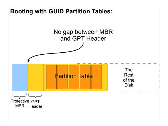
With GPT, there's still an MBR at the front of the disk (the MBR's partition table just says there's one big partition on the disk, of type "GPT"), but there's no "Compatibility gap" after this MBR. The GPT header is written right after the MBR. Where can we put the stage 1.5 bootloader now?
