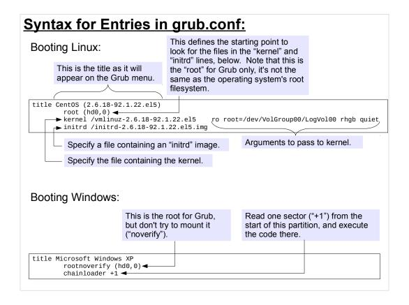
The Windows bootloader is embedded in the "partition boot sector" at the beginning of the partition on which Windows is installed. The second example above shows how Grub can just hand off the boot process to the Windows bootloader.
