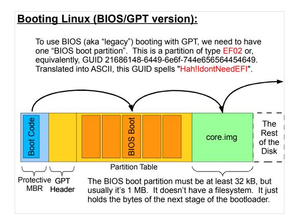
Instead of putting the "stage1.5" bootloader into the DOS compatibility region, we now need to make a separate small partition for it. Instead of "stage1.5", grub now calls this "core.img".
