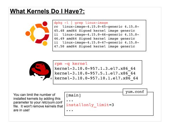
Installed kernels show up automatically in the boot menus generated by grub-mkconfig. The "installonly\_limit" option available in the RedHat/CentOS/Fedora world helps keep these menus uncluttered.
