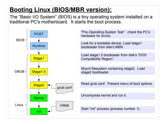
Grub (the "GRand Unified Bootloader") is the successor to the original Linux boot system, called LILO. With LILO, any time you made a change to the boot configuration, the bootloader needed to be re-installed in the disk's Master Boot Record (MBR). Grub understands filesystems, though, so you an reconfigure it by simply editing a text file that Grub's "stage2" will read when you reboot.
