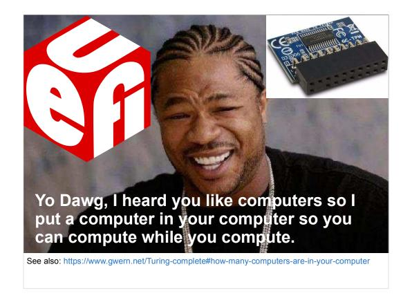
The UEFI processor, the TPM, and many other devices in your computer are actually turing-complete processors, capable of doing arbitrary calculations. The article linked to above finds that typical computers contain from 15 to several hundred processors or various kinds, including those found in network cards, disks, graphics cards, and even more unlikely places.
