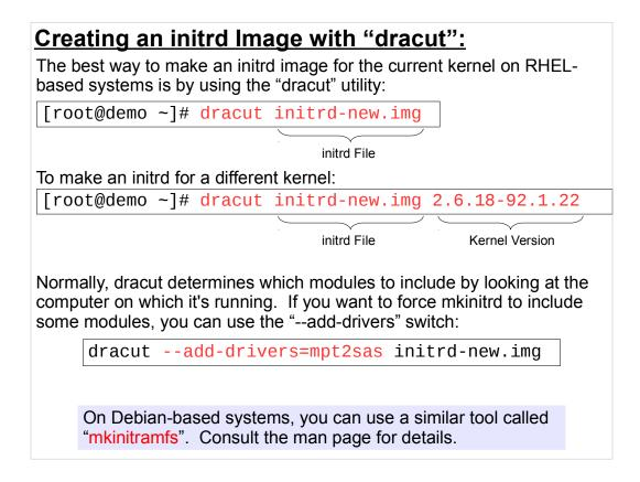
A given initrd will only work with one version of the kernel, because kernel modules are generally tied to a particular kernel version. dracut needs to know the intended kernel version so it can pack up appropriate modules.
