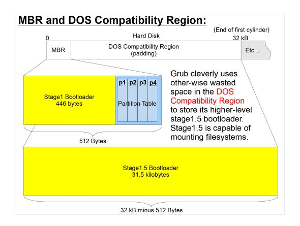
Some operating systems, like DOS, require that partitions start at cylinder boundaries in the C,H,S coordinate system. To accomodate this, most partition managers leave some padding between the MBR and the beginning of the first partition. This padding is called the "DOS Compatibility Region". On most disks, its size will be 32kB minus the 512 bytes needed for the MBR.
