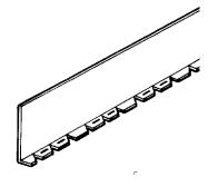
Figure 4.40 BARRIER STRIP-HORIZONTAL FITTING
