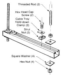
Figure 4.1F STRUT-EXPLODED VIEW
