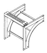
Figure 4.30 VERTICAL CABLE SUPPORT
