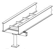
Figure 4.8A ELEVATED STRUT TYPE SUPPORT
