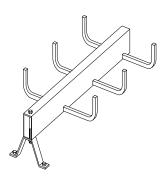
Figure 4.8C SINGLE RAIL FLOOR SUPPORT
