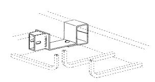
Figure 4.21A HORIZONTAL TEE OR 90° CONNECTOR
