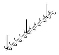
Figure 4.6A MULTIPLE SPLICE SUPPORT
