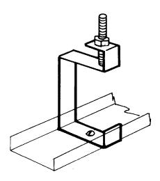
Figure 4.4 SINGLE CHANNEL HANGER
