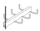
Figure 4.6B ROD THROUGH SPINE HANGER
