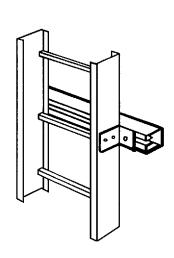
Figure 4.9C VERTICAL STRUT SUPPORT
