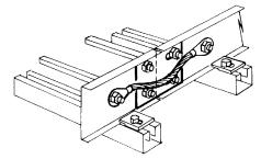
Figure 4.12 EXPANSION SPLICE PLATE ATTACHMENT
