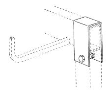
Figure 4.21D **VERTICAL TEE OR 90° CONNECTOR**
