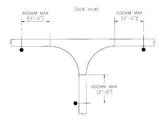
Figure 4.28 VERTICAL TEE (Side View)
