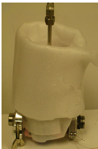
Figure A.6: Photo of the liquid nitrogen cooled fiber housing. Note the styrofoam used from insulation.
