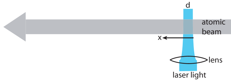
Figure 5.1: Schematic of laser light focused into the potassium atomic beam exciting a cylinder of Rydberg atoms with a Gaussian profile. The atoms spread due to their thermal velocity distribution, so the average relative speed between neighboring Rydberg atoms is reduced.
