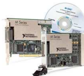
Figure 6. Two different packages – one software standard. In software, communication with a PXI module (bottom) is identical to that with a PCI board (top).
