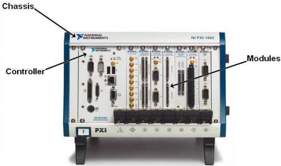
Figure 1. A standard 8-Slot PXI chassis contains an embedded system controller and seven peripheral modules.
