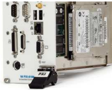
Figure 5. National Instruments PXI-8187 Pentium 4-M 2.5 GHz Embedded Controller. Notice the familiar PC peripherals such as keyboard/mouse and monitor connections, as well as the hard drive, USB 2.0, Ethernet, serial, and other standard PC peripherals. This controller runs standard Windows 2000/XP OSs, or can be targeted with LabVIEW Real-Time.
