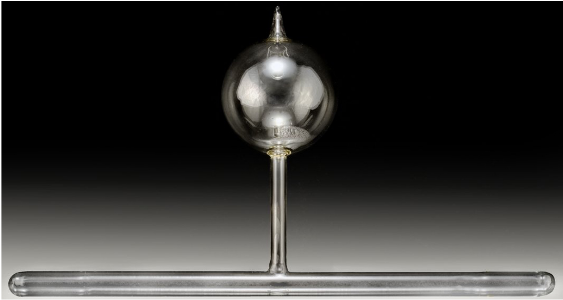
Figure 1.9: SEOP Polarized Target Cell Used for G_E^n (E02013). Image provided by Al Gavalya.
