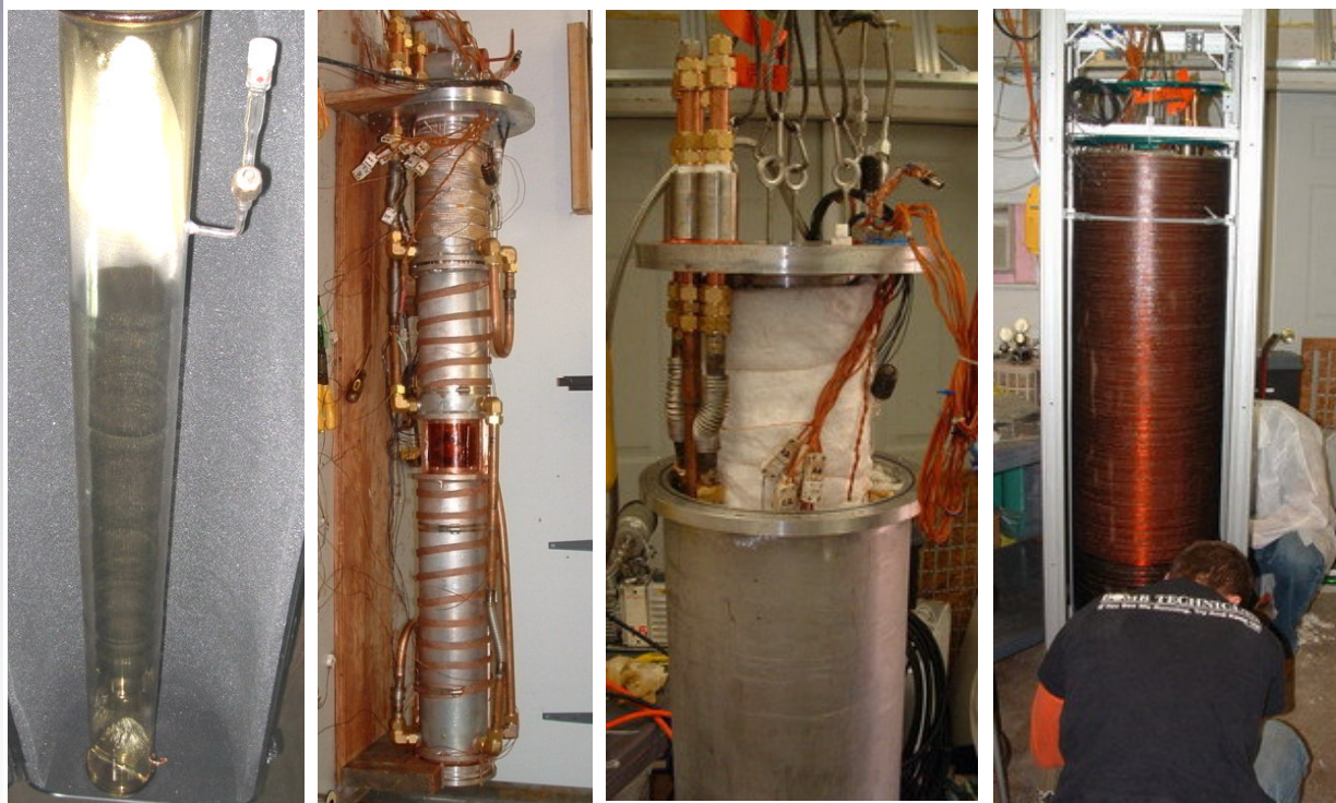
Cartridge with cell and oven, to be loaded in pressure vessel.
