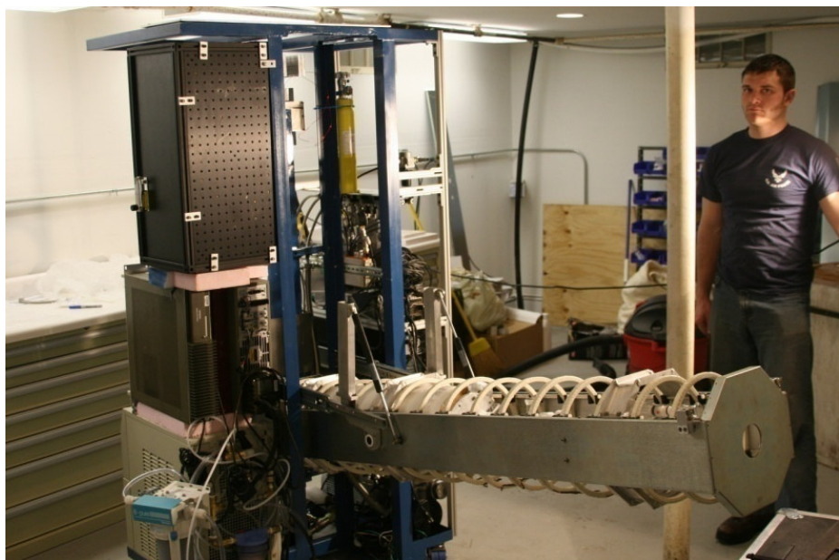
“Bell” system. Column replacement position (left). Operational system (right) including motorized freeze-out.
