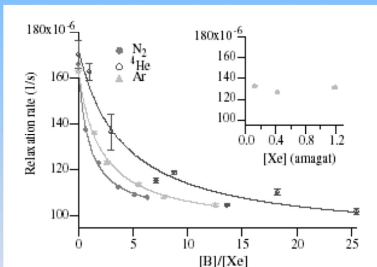
FIG. 1. Xe spin-relaxation rate as a function of composition, for various buffer gases, at a fixed Xe density of 0.15 amagat. Inset: Relaxation rate for  $[\text{Ar}]/[\text{Xe}] = 1.75$  as a function of Xe density.
