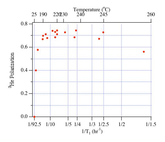
Very fast (2.5 hrs), high polarization (76%) w/ only 12 W pumping power
