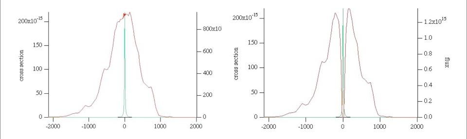
Spectral hole quickly reduces optical pumping rate at front of cell, thus reducing Rb polarization.
