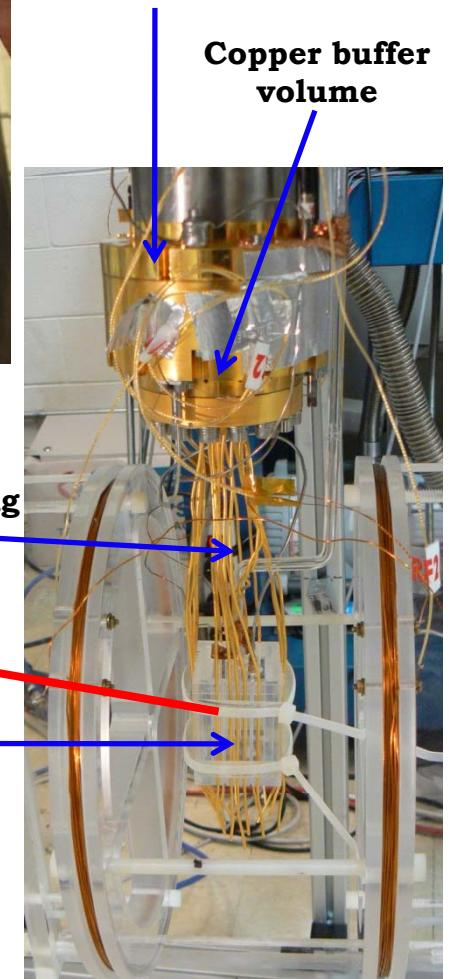
**Copper cooling wires**
