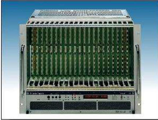
21 slot 6U crate for 19" racks
