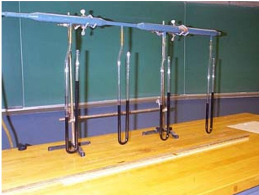
The difference in heights of the dark liquid in the two arms of the U-tubes measures the pressure difference between that point in the flow tube and the outside atmospheric pressure.
