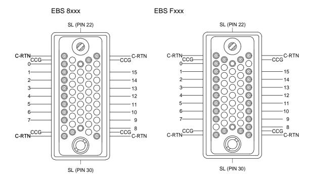
CCG is connected with the Crate-GND and the shield
